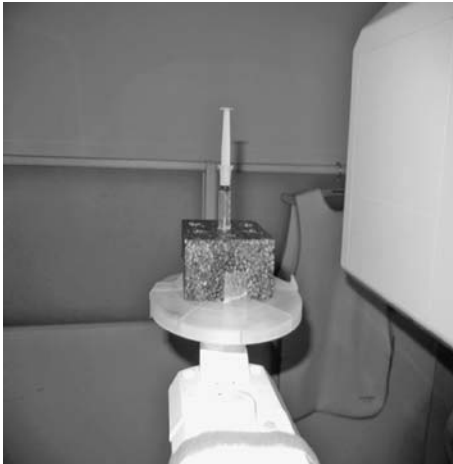
Fig. 2 Placement of a test sample in the center of the FOV for CBCT.
