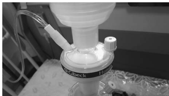
Fig. 2 Injection apparatus. A 2% methylcellulose solution injected through the injection port spreads across the surface of the paper filter inside the heat and moisture exchange filter.
