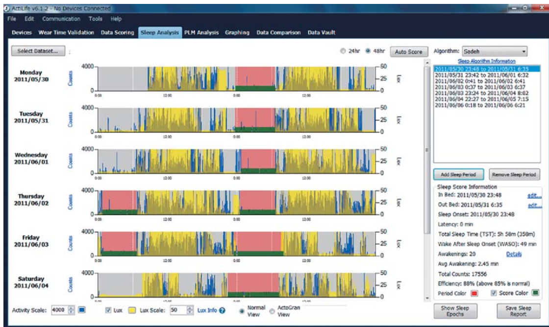
Fig. 3 Sleep analysis screen of ActiLife (ActiGraph, Pensacola, FL, USA). Screen displays six graphs where the raw activity data, illuminance and analyzed sleep time of 48 hours were shown. Algorithm is shown in the upper-right corner. Sleep scores are shown in the lower-right corner. Blue : Activity, Pink : In bed, Green : Sleep, Yellow : Illuminance.
