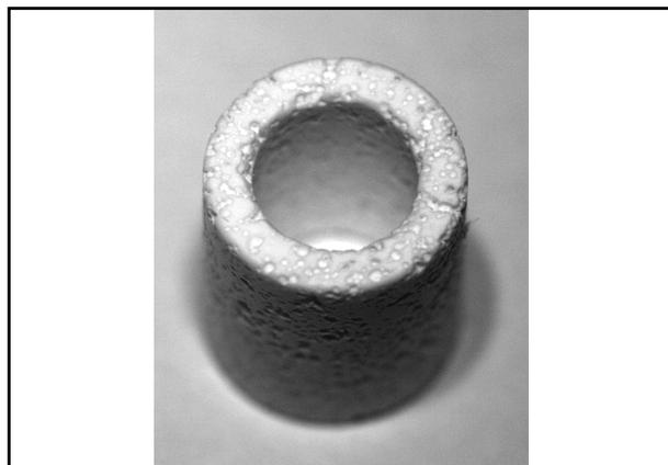
**Figure 1.** Macro-photographic image of cylindrical porous hydroxyapatite with a hollow center (10 mm in height, 8 mm in outer diameter, and 5 mm in the hollow center). Total porosity was 55%. The diameter of the aperture between interconnected pores was approximately 50 - 300  $\mu\text{m}$ .
